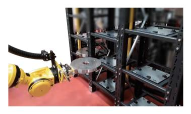
Pallet-Transfer Automation with Articulated Robot
