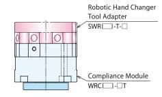
(ex.) In case of using WRC0070-2T with Robotic Hand Changer: WRC0070-2T can be directly mounted on the tool adapter of Robotic Hand Changer: SWR0070-T-.
