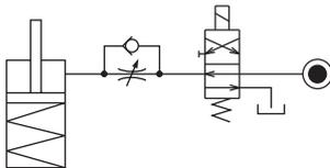
If the cylinder may be damaged by the load from the releasing action direction, provide the flow control valve to the releasing side as well. (Provide the flow control valve to the releasing side if the lever weight is applied during release action.)
