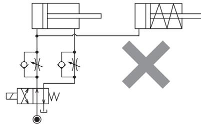
Refer to the following circuit when both the single acting cylinder and double acting cylinder are used together.
