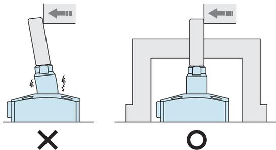
When clamping workpieces of different heights
