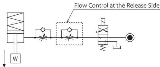
● Speed Control Circuit for Double Acting Cylinder
