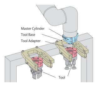
High-precision robotic hand changer enables a robot to perform multiple operations.
