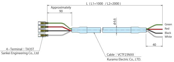
Conductor Cross-Sectional Area: 0.5mm<sup>2</sup> (AWG20)
