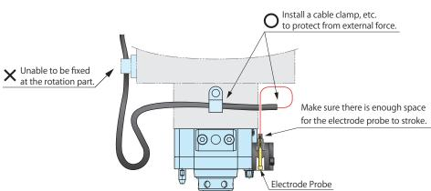
As for Compact Electric Power Transmission option, the electrode probes on both master cylinder and tool adapter are exchangeable.
